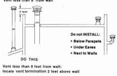
Figure 5. Termination Height Requirements.
